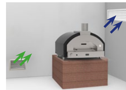
➔ NATURAL VENTILATION - S=300cm 2 ➔ NATURAL AERATION - S>100cm 2
